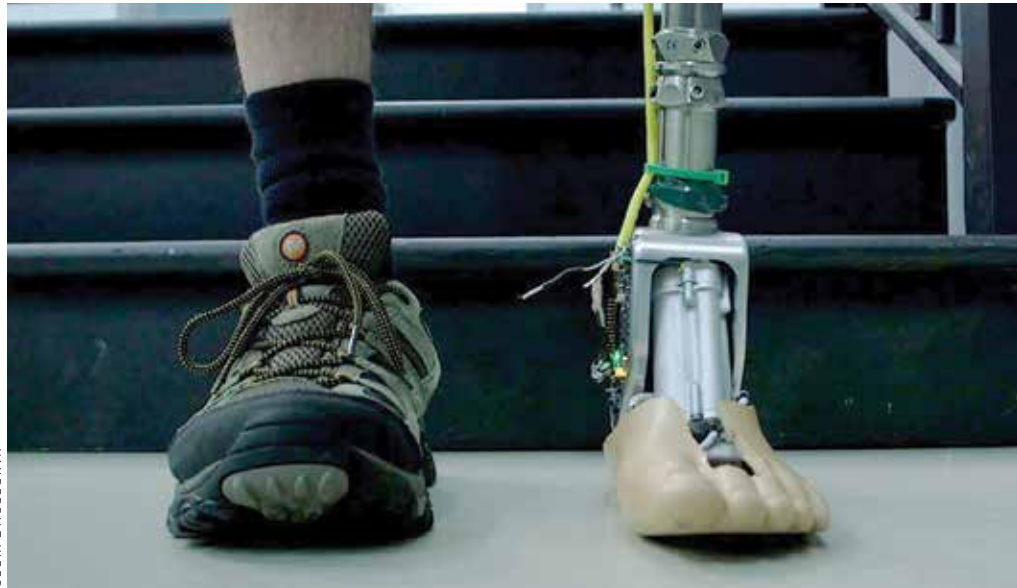
Unlike static prosthetic ankles now available for amputees, the new intelligent ankle from Michael Goldfarb's lab anticipates the user's movement and adjusts the feet to different terrains, thanks to a tiny motor, actuator, sensors and a microchip.
